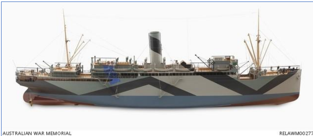
A 1/30 scale full hull shipbuilder's model of H.M.A.T. 'Warilda', painted to represent its service as an Ambulance Transport, with sawtooth dazzle camouflage.
